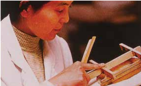
3 日本の竹枠に似た竹刀で箔を切り揃える (同上パンフレットより) 3 The finished gold leaf is cut with a bamboo square framed cutter, similar to that used in Japan. (Source: Nanjing Gold Leaf Company Pamphlet)
