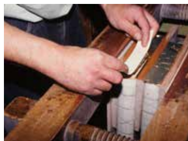
6 天金を施す (フィレンツェ) 6 Gilding the top edge of books. (Florence)
