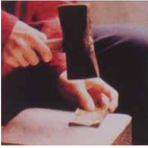
1 延金を、紙を間に挟まずに、 40~50枚重ねて打つ (南京金箔公司パンフレットより) 1 Sheets of gold are beaten in layers of up to 40-50 sheets together without being separated by papers. (Source: Nanjing Gold Leaf Company Pamphlet)
