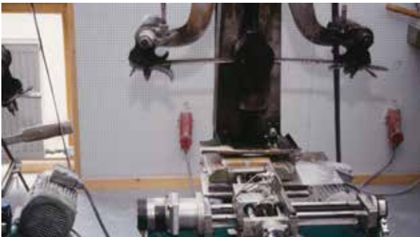
2 シリンダーを受ける台座を可動式に改良した箔打機(同上) 2 An improved hammering machine that has a flexible, movable tray that allows the beating cylinder to be fixed. (Gerstendörfer, Germany)
