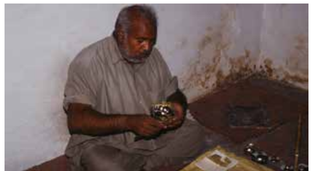
7 銅製のボディに水銀を素手で塗るカラシュ職人 (同上) 7 A kalash craftsman who coats mercury on to a copper body using his hands that are unprotected. (Jaipur)
