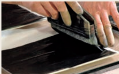
Factory-made glassine paper is coated with carbon (plant soot), aluminum powder, casein, and a surfactant.
